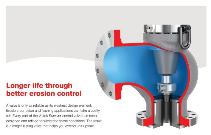
Valtek Survivor valve cutaway depicting standard seat with ceramic plug and seat inserts
