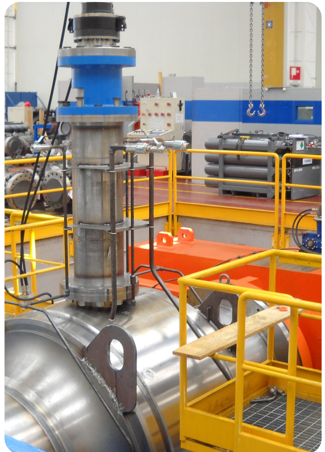
In-house testing facilities for valves up to 1600 mm (64")
