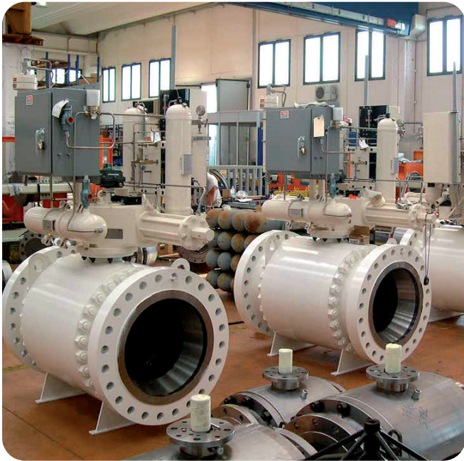
Actuated valves for testing in the in-house valve automation centre
