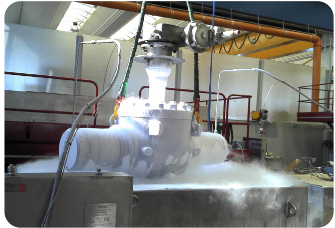
Cryogenic testing on a 16" (400 mm) Class 1500 Top Entry Ball Valve
