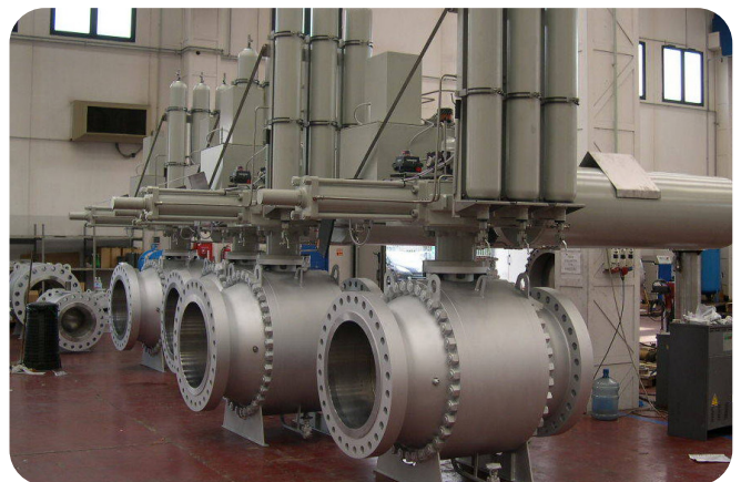
24" (600 mm) Class 1500 Ball Valves with Gas Over Oil actuators
