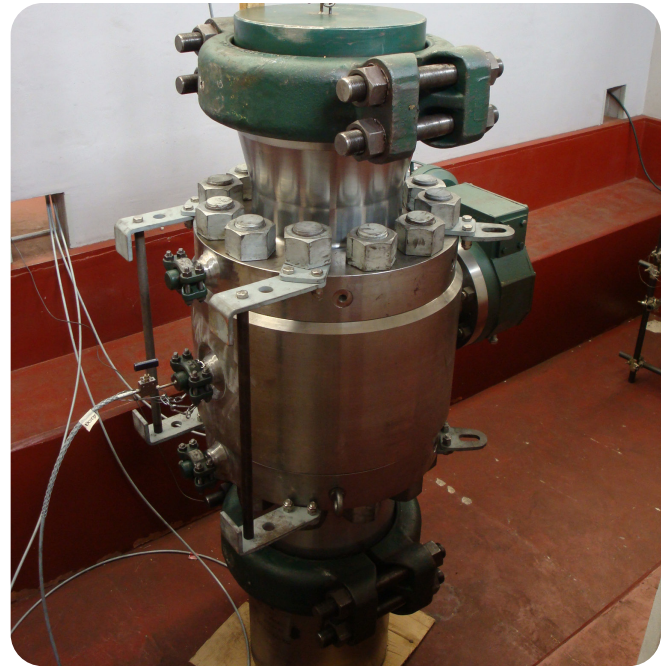
Hydraulic Shell & Seat Test on a 18" (450 mm) Class 2500 Uprated valve
