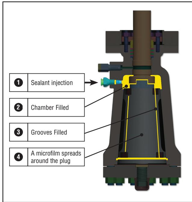
Sealants should be selected based on service media and operating temperature. The tables below summarize our general sealant recommendations. Sealant should be carefully selected since the use of the correct Serck Audco Sealant will minimize injection frequency. The tables are self explanatory, however, if in doubt regarding sealant selection, Serck Audco can suggest a suitable sealant against service details.
