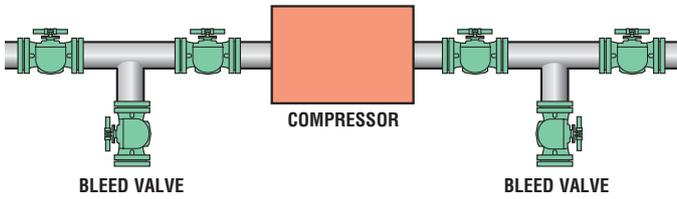
Configuration using double isolation plug valves
