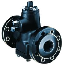
A high pressure plug valve, achieving exceptional reliability on both leak tightness and operability. The valve ensures long-term line and atmospheric sealing, minimizes routine maintenance, and is fire tested to API6FA.
