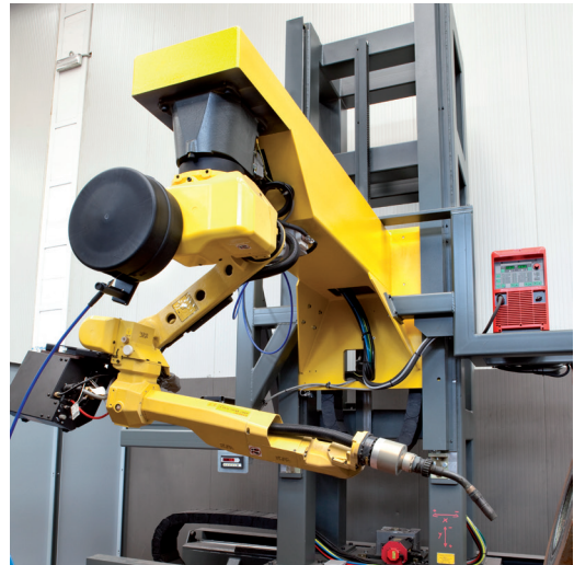
SAW welding robot applying weld overlay on valve closure
