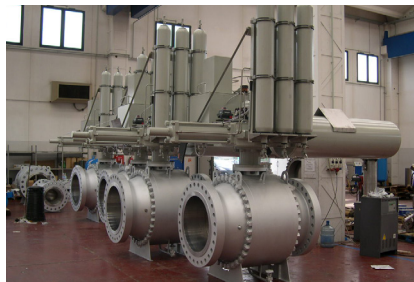
24" (600 mm) Class 1500 Ball Valves with Gas Over Oil actuators
