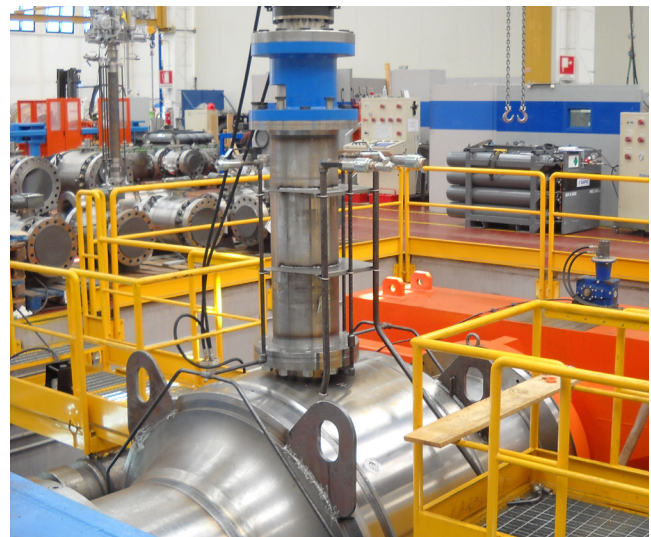
In-house testing facilities for valves up to 1600 mm (64" )
