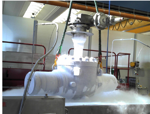
Cryogenic testing on a 16" (400 mm) Class 1500 Top Entry Ball Valve
