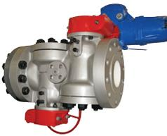
DIPV gives all the advantages of our pressure balanced plug valve but also provides a double block and bleed system with true double isolation and two independent obturators in an extremely compact form. In the DIPV, the plugs are mounted in inverse orientation to obtain the maximum port area
