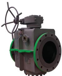
For all applications where the media needs to be maintained at elevated temperatures and metal to metal seats are required, such as molten sulphur, the SAV steam jacketed plug valve provides the best solution. Also suitable for high pressures, it will be supplied with oversized flanges for full jacket option.
