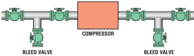
Configuration using twin isolation plug valves
