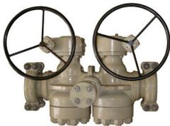
TIPV gives all the advantages of our pressure balanced plug valve but also provides a double block and bleed system with true double isolation and two independent obturators in an extremely compact form. In the TIPV, the plugs are mounted in same orientation to facilitate installation on particular plant layouts
